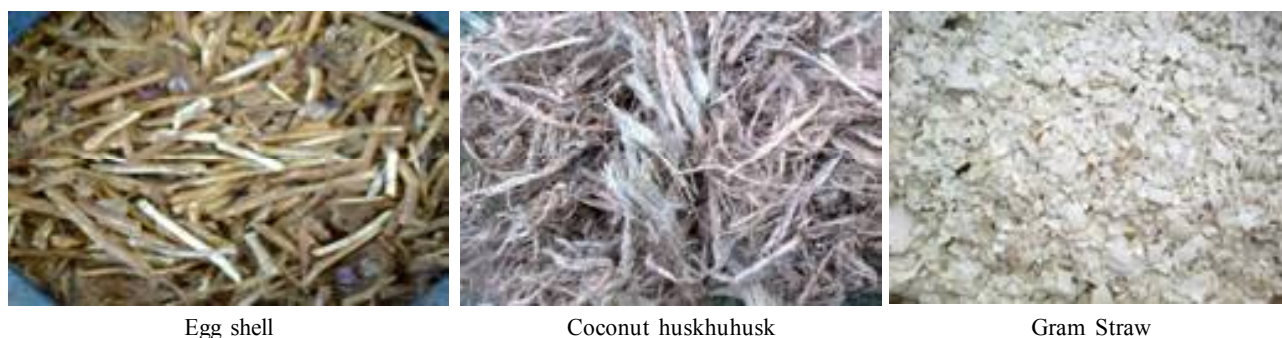
Fig. 2. Pictorial view of organic filters component
